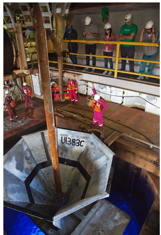
Reentry cones like the one pictured here will be deployed at the South Atlantic Transect boreholes during the current engineering Expedition 390C. Image credit William Crawford, IODP JRSO.
