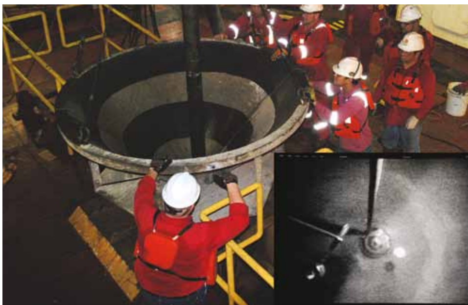
Figure 3—Preparing for hole re-entry at Site U1347 after the bit-change. The crew is about to drop the free-fall funnel through the moon pool and down to the seafloor over 3 km below the boat. The pipe is then pulled up and a new drill bit attached to the end. The drill string is then lowered back into the water and the hole is re-entered with the aid of the funnel and a grainy black-and-white camera image of the seafloor (inset image). Photo credit Will Sager.
