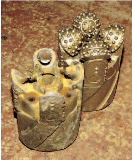
Figure 3. Photograph showing used C-7 bit missing all of its cones. Note a small fragment of one cone remains. New C-7 bit shown for comparison.
