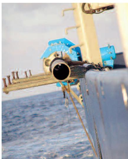
Figure 5. Sediment piston corer before deployment (in horizontal orientation). The empty tubing is lowered vertically on a steel wire to the sea-floor at approximately 5km depth, before capturing approximately 14m of sediment from the upper part of the sea-floor. Coring operations were performed by a crew from Oregon State University onboard the R/V Roger Revelle.
