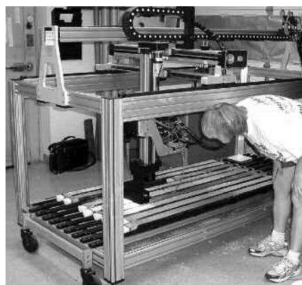
Figure 1. MSCL-XYZ system set up for RGB linescan imaging of archive core.
